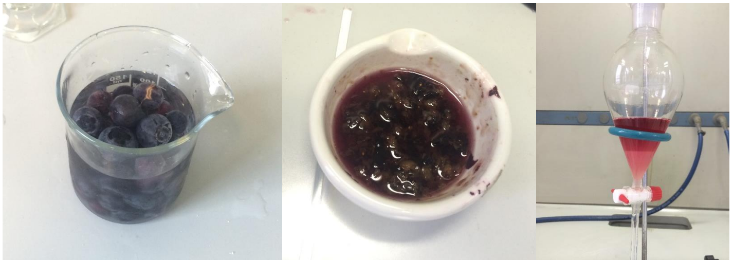
Ptc. 4) Blueberries in a diluted acetic acid solution, blueberries in acetone and phase separation extraction with petroleum ether (from left to right).
