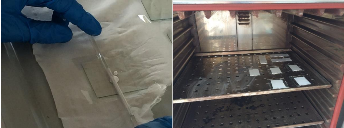
Ptc. 6) The preparation of the TiO_2 surface on conductive glass.
